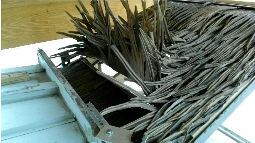
Representative Photograph Deck #1: One leaf has disengaged from rail at 29 minutes into testing at 130mph
